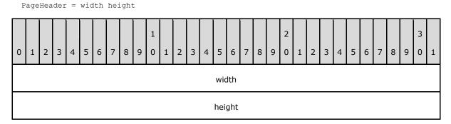
width (4 bytes): A Float value field that specifies the width, in millimeters, of a physical page of the report, including the margins. The value of this field MUST be a non-negative Float.  $\leq 1 \geq 1$
