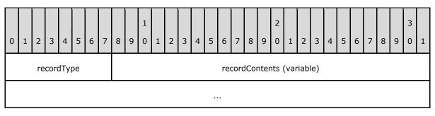
[MS-RGDI] — v20100903 Remote GDI+ (RGDI) Binary Stream Format Structure Specification
