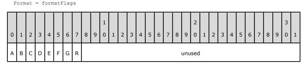
formatFlags (1 byte): A byte field that specifies the formatting to be applied when drawing a string. The format flags are a combination of the following basic formatting properties: Vertical Writing Mode, RTL Direction, Character Trim, Bottom Alignment, Top Alignment, Right Alignment, and Left Alignment. This field is a bitmask and is specified by the following bit fields:
