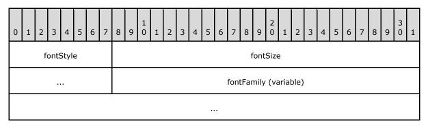
**fontStyle (1 byte):** A byte field that specifies the style of the font. The font style is a combination of the following basic font styles: **Strikeout**, **Underline**, **Bold**, and **Italic**. This field is a bitmask and is specified by the following bit fields.
