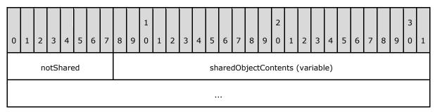
**notShared (1 byte):** A byte field that specifies that the type of the <u>ShareableObject</u> structure is a **NonSharedObject** structure. The value of this field MUST be "0x00".
