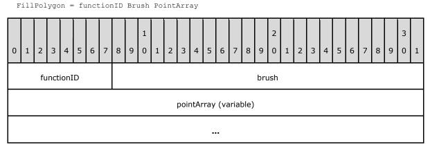
**functionID (1 byte):** A byte field that specifies that the type of the function is **FillPolygon**. The value of this field MUST be "0x04".
