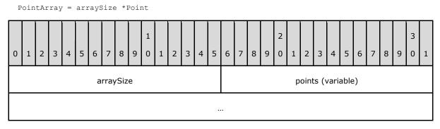
arraySize (2 bytes): A UInt16 value that specifies the number of <u>Point</u> structures in the array.
