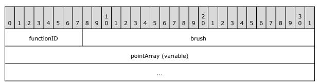
**functionID (1 byte):** A byte field that specifies that the type of the function is **FillPolygon**. The value of this field MUST be "0x04".
