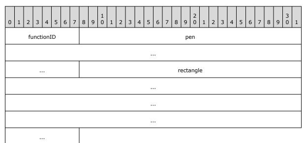
**functionID (1 byte):** A byte field that specifies that the type of the function is **DrawRectangle**. The value of this field MUST be "0x01".
