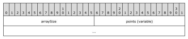
arraySize (2 bytes): A UInt16 value that specifies the number of <u>Point</u> structures in the array.
