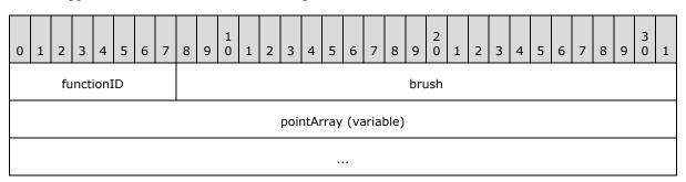
**functionID (1 byte):** A byte field that specifies that the type of the function is **FillPolygon**. The value of this field MUST be "0x04".
