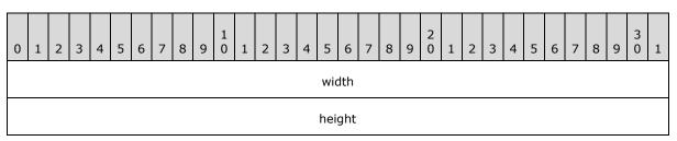
width (4 bytes): A Float value field that specifies the width, in millimeters, of a physical page of the report, including the margins. The value of this field MUST be a non-negative Float.
