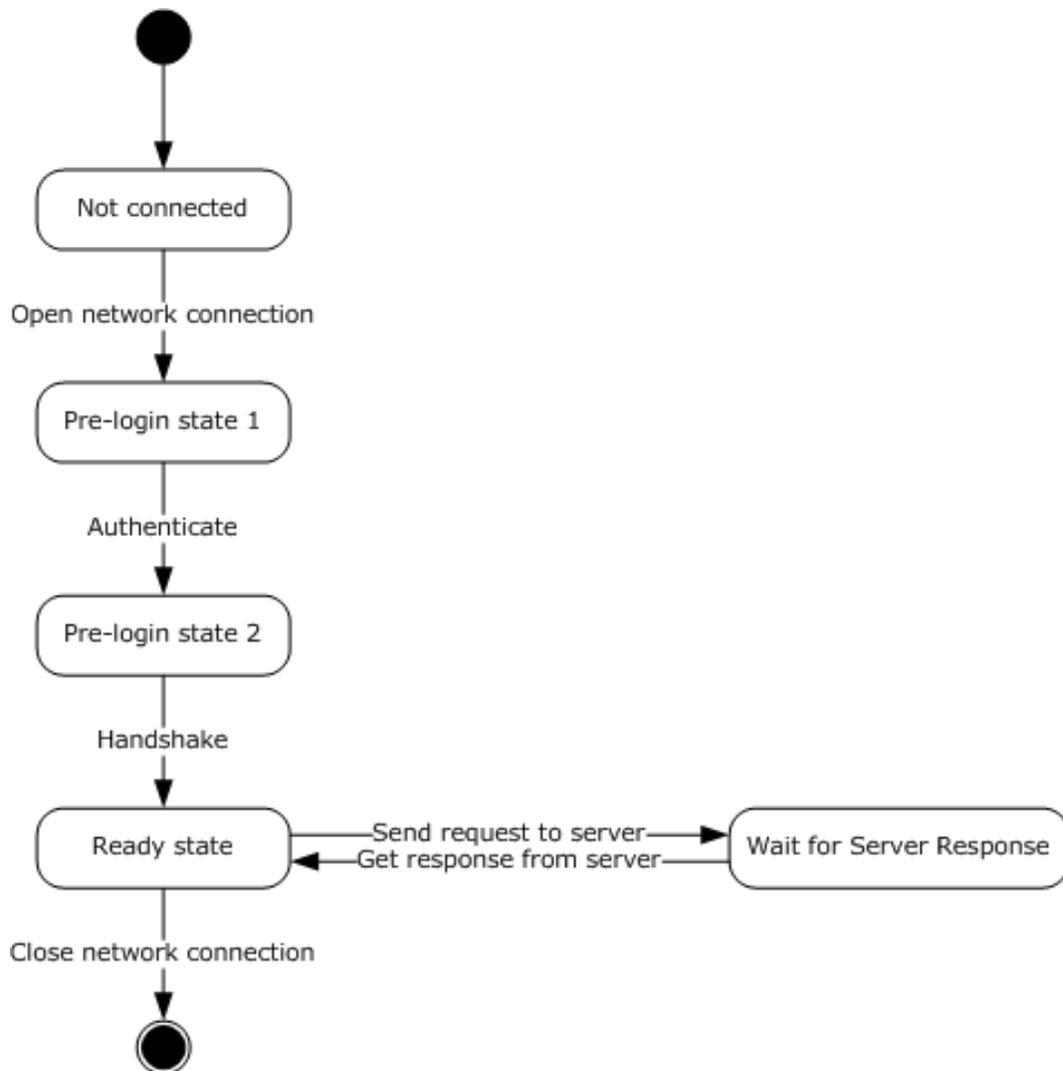
**Figure 4: Client connection state diagram (client perspective)**
